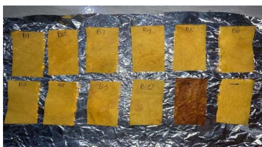
Figure 1. Test results for borax using tumeric paper
