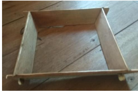
Figure 3. Frame of the Sagu Sieve made from pule wood
