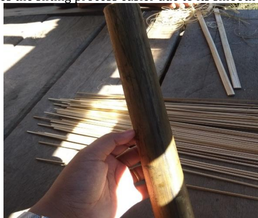
Figure 4. Bamboo as the filter material of the Sagu Sieve
