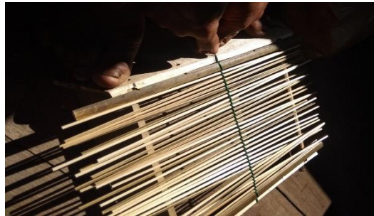
Figure 4. Process of binding bamboo for the Sagu Sieve filter
